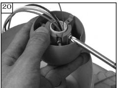
Tighten set screw to hold ball in place.
